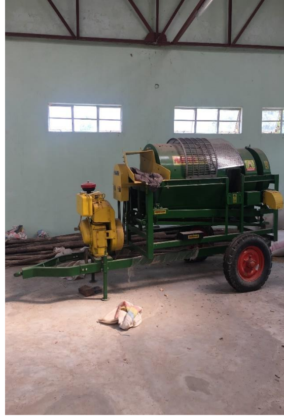
Figure 1 Groundnut Sheller and Multi crop thresher that require a tractor for pulling
