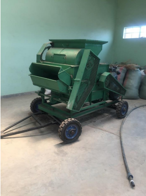
Figure 1 Groundnut Sheller and Multi crop thresher that require a tractor for pulling
